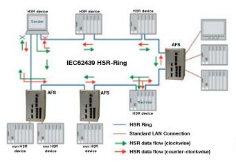
Duplicate data packets are transmitted simultaneously in both directions
