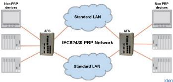
Identical data packets are transmitted simultaneously to both networks
